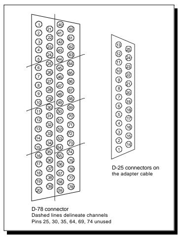
Figure 19 --- ESC-100D Output Connectors
